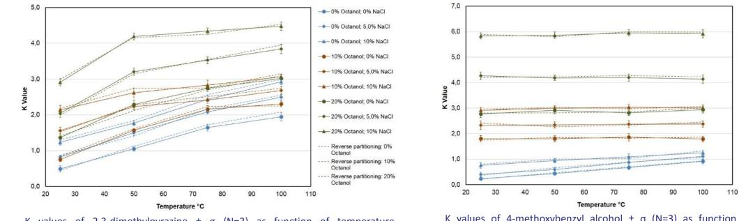
K values of 2,3-dimethylpyrazine  $\pm \sigma$  (N=3) as function of temperature, composition of the hydrocarbon phase and salinity
