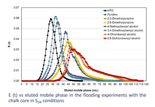
• The partitioning tracer candidates are delayed relatively to HTO
