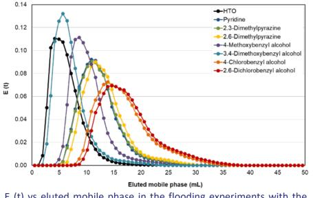
E (t) vs eluted mobile phase in the flooding experiments with the sandstone core in  $S_{\mbox{\scriptsize OR}}$  conditions
