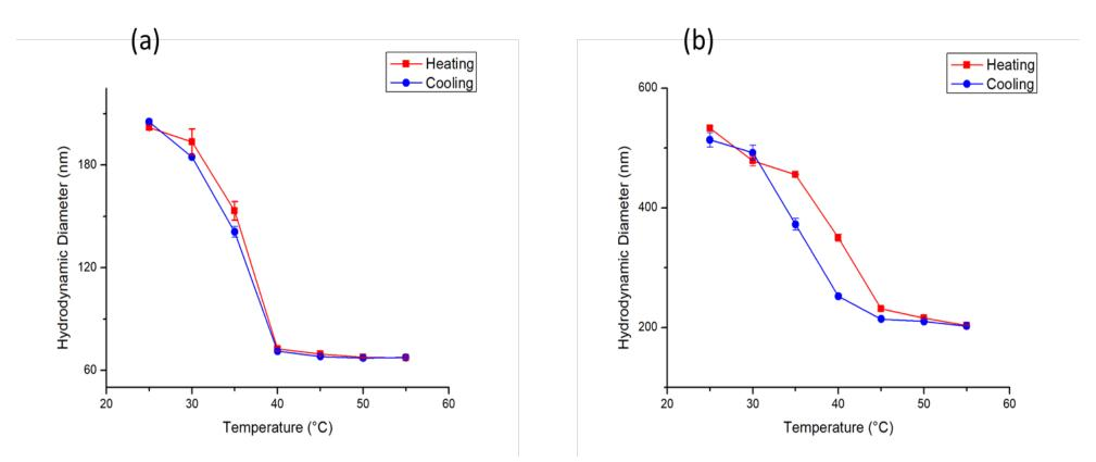
Figure: Reversible swelling and collapse of the nanogels as function of the temperature: (a) NG01 and (b) NG05
