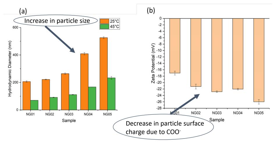
Figure: (a) Hydrodynamic diameter at swelled and collapsed state of different nanogel samples of varying mole ratios of NIPAm and AAc. (b) Zeta potential measurements of various nanogel samples.
