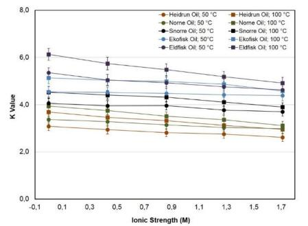
K value of 2,6-dichlorobenzyl alcohol to 5 different crude oils as function of the ionic strength of the aqueous phase at 50  $^\circ$ C and 100  $^\circ$ C.
