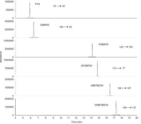
Reconstructed SRM chromatogram of produced water from Ekofisk M spiked at 1  $\mu$ g L<sup>-1</sup> with the tracer candidates.
