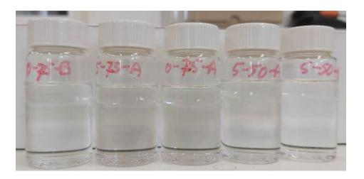
Brines with ionic strength (I) between 0 – 1,71 M were used. Divalent vs monovalent ions were also evaluated.
