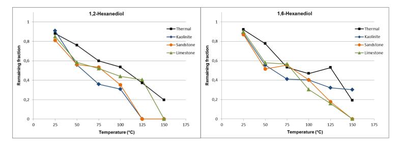
• RF of 1,2 and 1,6-hexanediol as a function of temperature after 12 weeks with and without rock substrates.
