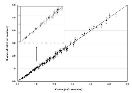
K values  $\pm \sigma$  (N=3) of the tested compounds in experiments with an aqueous phase containing divalent ions vs the K values in experiments with an aqueous phase containing only NaCl.
