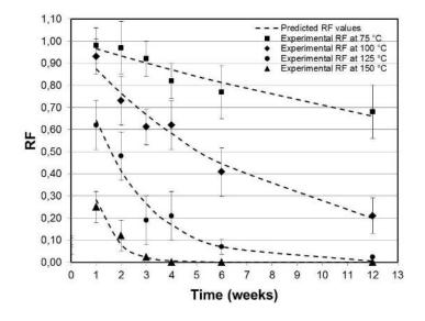
Experimental vs predicted RF values of 4-hydroxybenzyl alcohol (paper III)
