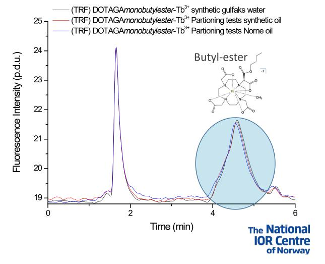
**Tracer exclusively hydrophilic !** Despite of the retention on the  $C_{18}$  column
