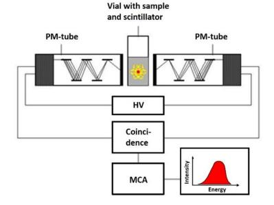
Simplified liquid scintillation counter scheme
