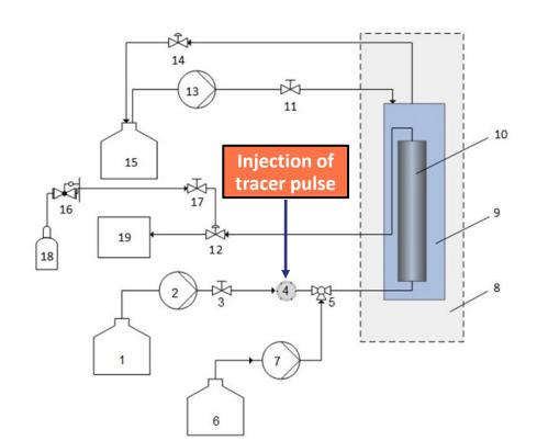
Scheme of the experimental setup used in the flooding experiments
