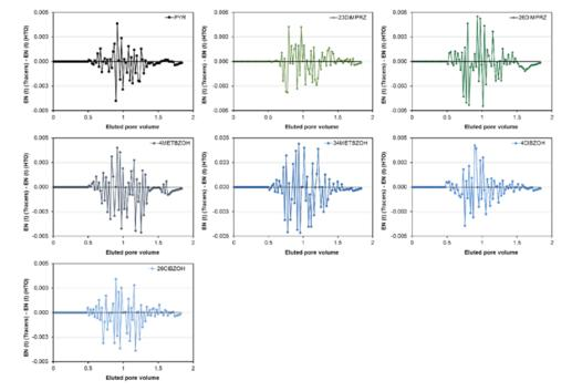
EN (t) of the PITT tracer candidates – EN (t) of HTO vs eluted pore volume in the water saturated chalk core.
