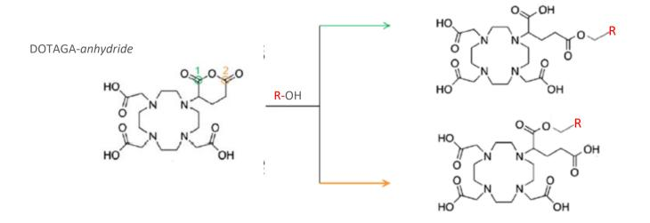
By varying R length  $\rightarrow$  partitionning coefficient adjustement (K<sub>part.</sub>)
