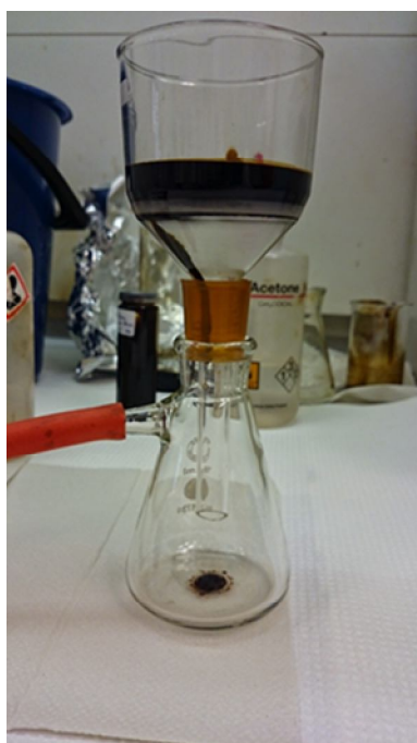
Figure 5.4.1.1: Filtration of crude oil emulsion (w/o) through filter 4 with pore size 10 - 16 \mu\text{m} . It looked like the first part passing the filter contained a large amount of water.
