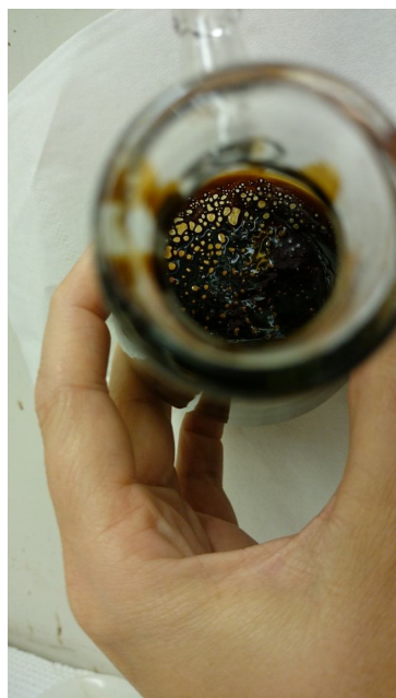
Figure 5.4.1.3: Filtration of crude oil emulsion (w/o) through filter 4 with pore size 10 - 16 \mu\text{m} . The picture shows the water droplets in the bottom of the Erlenmeyer flask after removing a part of the sample for NMR.
