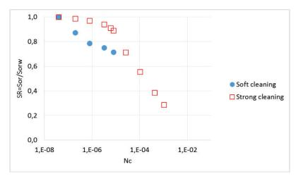
Figure 4 Capillary Desaturation Curve (CDC), normalized residual saturation vs capillary number (Sor/Sorw vs Nc) after methanol cleaning (soft) and after cleaning with methanol/toluene, acetic acid and ethanol cleaning (strong) of reservoir core (Fjelde et al., 2015).
