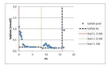
Figure 12 Production of sulphate from reservoir chalk by injecting desulphated sea water (D-SW) (Fjelde, 2018).
