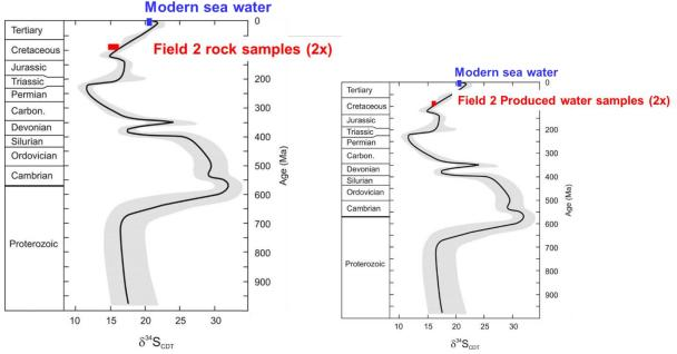
Figure 10 Sulphur isotopic ratio ( $\delta^{34}S_{CDT}$ ) for BaSO<sub>4</sub>-filtercakes precipitated from dissolved Field 2 rock and from produced water samples compared to modern sea water samples (Fjelde, 2019).
