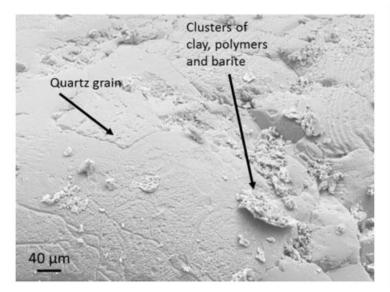
*Figure 6 Detection of mud additives by SEM and EDAX on a core slice after water flooding (Fjelde et al., 2015).*
