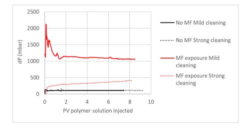
Figure 7 Differential pressure (dP) during polymer flooding experiments using core plugs with and without mud filtrate contamination. The core plugs were prepared by either mild cleaning (STO injection) or strong cleaning (toluene/methanol cycles) (Fjelde, 2022b).
