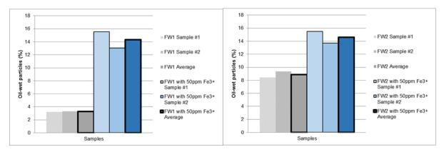
Figure 13 Concentration of oil-wet particles in flotation experiments with Glauconite and STO and two different formation waters (FW1 and FW2) (Fjelde et al., 2017b).
