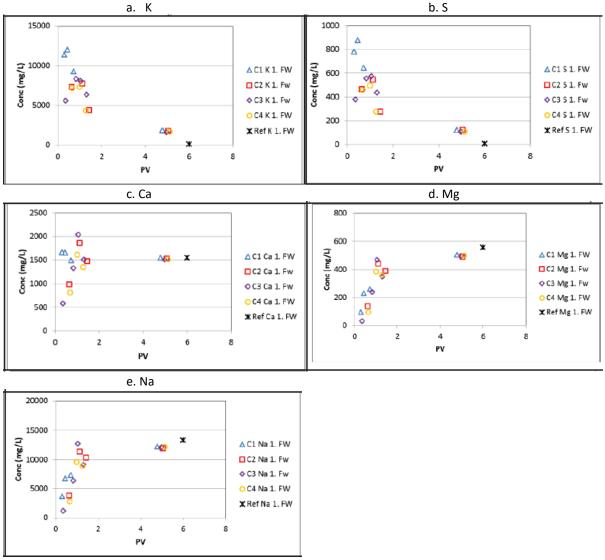
*Figure 5 Effluent element concentrations during SFW injection before solvent cleaning of four core plugs (Fjelde et al., 2015).*
