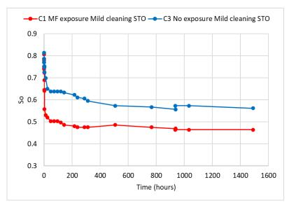
Figure 3 Spontaneous imbibition of formation water at  $60^{\circ}C$  for core plug exposed to mud filtrate from OBM without asphalt product (C1 MF exposure Mild cleaning) and core plug not exposed (C3 No exposure Mild cleaning STO), both core plugs were cleaned by injection of STO at S<sub>wi</sub> (Fjelde, 2022a).
