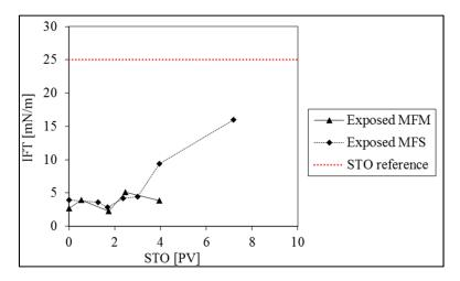
Figure 1 Interfacial tension between effluent and water during injection of stock tank oil to sandstone core plugs exposed to mud filtrate of OBM containing asphalt product, MFM = Mud Filtrate Mineral base oil and MFS = Mud Filtrate Synthetic base oil. STO was injected instead of mud filtrate to the reference core plug (Fjelde et al., 2015).
