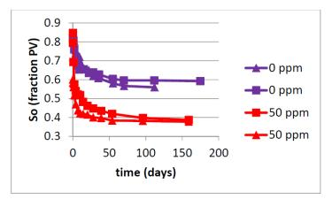
Figure 11 Oil saturation (So) vs time during spontaneous imbibition of sea water into core plugs prepared by formation water with (50ppm) and without (0ppm) sulphate (Fjelde and Asen, 2015).
