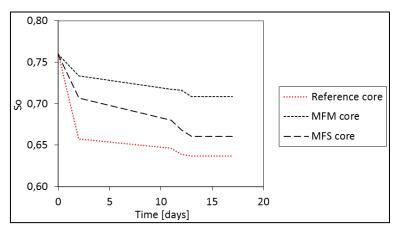
Figure 2 Spontaneous imbibition of formation water for core plugs exposed to mud filtrates from OBM containing asphalt product (MFM and MFS: Mud filtrates with mineral and synthetic base oils) and core plug not exposed (Reference core) (Fjelde et al., 2015).
