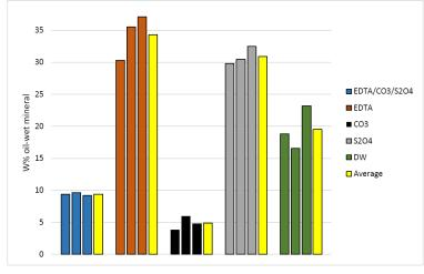
Figure 14 Concentration of oil-wet glauconite clay particles when exposed to chemical package and its components. CO3 = Sodium bicarbonate, S2O4=sodium dithionite, DW=diluted water (Magnussen, 2017).
