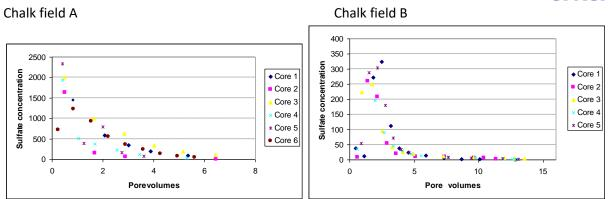
*Figure 8 Effluent sulphate concentration during injection of synthetic formation water without sulphate to reservoir chalk plugs from two fields (Fjelde, 2008).*
